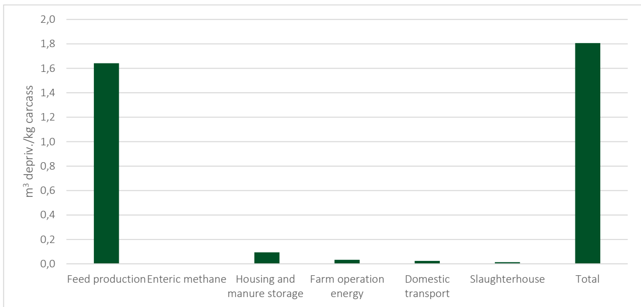
Figure 3.39 Water scarcity (m 3 depriv.) per kg carcass of turkey through the life cycle (cradle to slaughterhouse gate).
